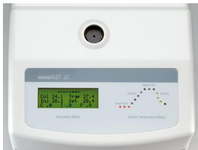
The microFAST™ GC Front Panel. Injection sampling port is shown at the top of the photo. Instrument status display is lower left. Column temperature LEDs are lower right.
