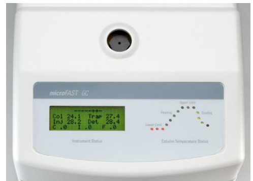
The microFAST™ GC Front Panel. Injection sampling port is shown at the top of the photo. Instrument status display is lower left. Column temperature LEDs are lower right.
